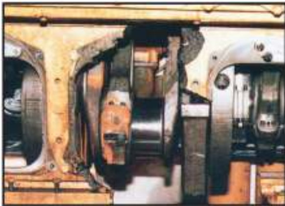
Figure 3 Damaged Core Refund Broken engine block
