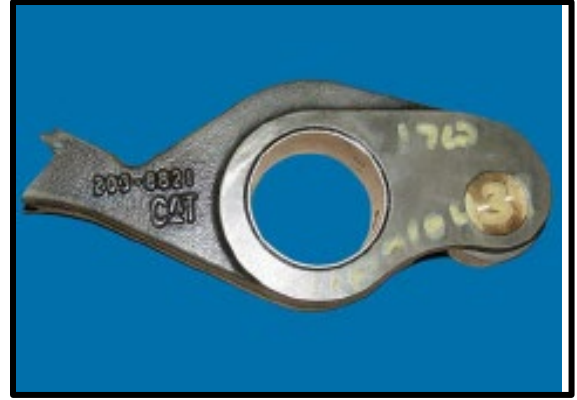
Figure 4 No Core Refund Broken forging
