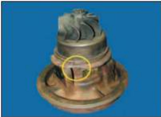
Figure 5: Non-operational damage - broken center housing
