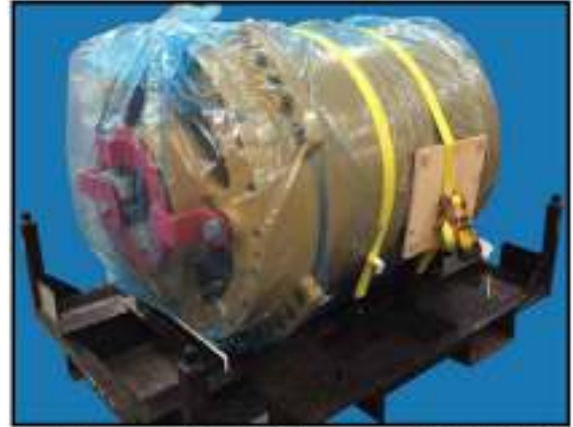
Figure 2 795 Traction Motor Full core Refund Properly wrapped and secured to the shipping stand (Material added behind Ratchet to avoid damage to wrapping)
