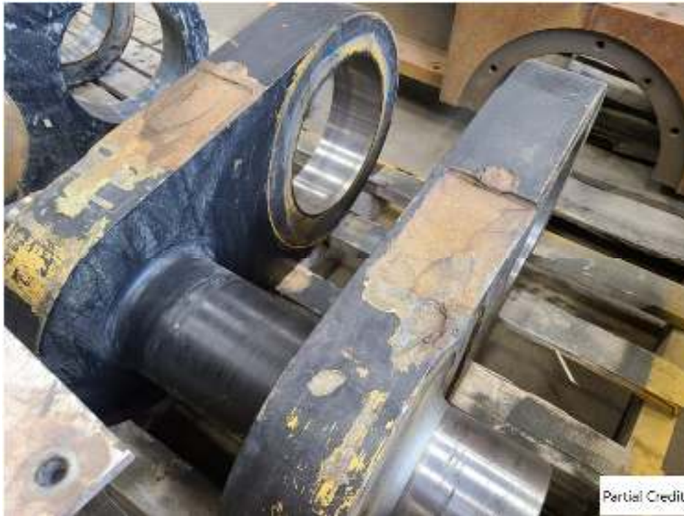
Figure 1 – There is evidence of pitting marks behind the normal wear surface of the link. This would be considered operational damage and would result in a partial credit.
