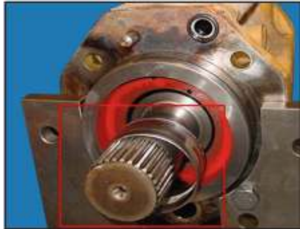
Figure 4: Shaft bearing failure
