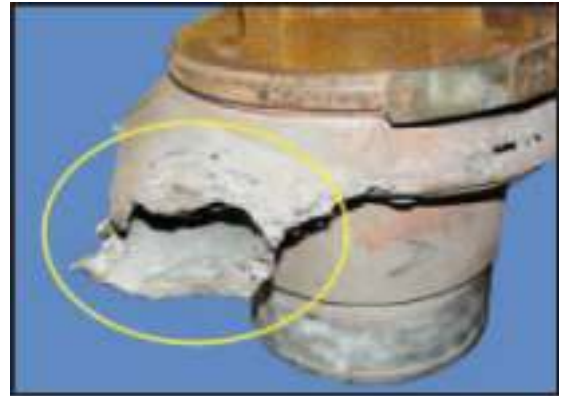
Figure 4: Turbocharger damaged by fire
