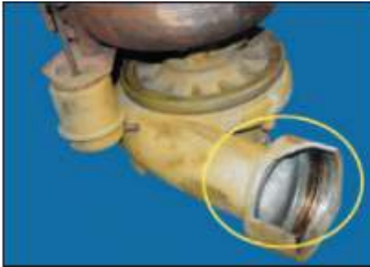
Figure 3: Broken housing resulting from mishandling
