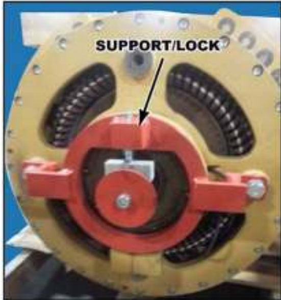
Figure 1 Full Core Refund Rotor shaft support/lock (Traction motor only)
