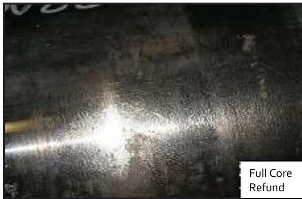
Figure 1: Spider web cracking on rod chromed surface.
