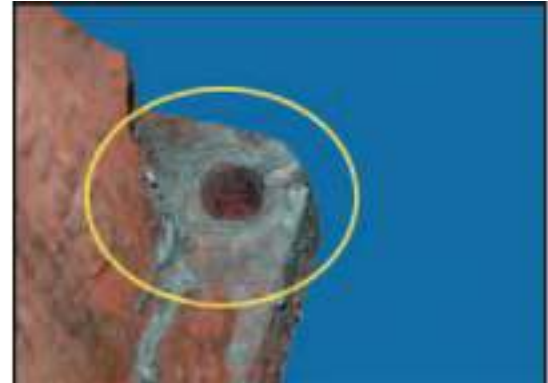
Figure 6: Non-operational damage - melted by torch
