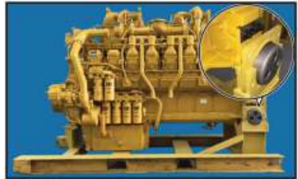
Figure 2 Full Core Refund Engine with rear mounts and modified stand
