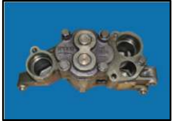
Figure 4 Core Refund Less Add Charge Missing retainer and spring
