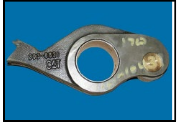
Figure 4 No Core Refund Broken forging
