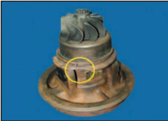
Figure 5: Non-operational damage - broken center housing
