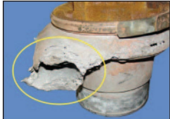
Figure 4: Turbocharger damaged by fire
