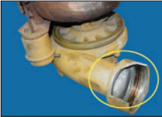
Figure 3: Broken housing resulting from mishandling
