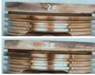
Minimal piston deposits after a proprietary 500-hour endurance test of Cat DEO-ULS.
